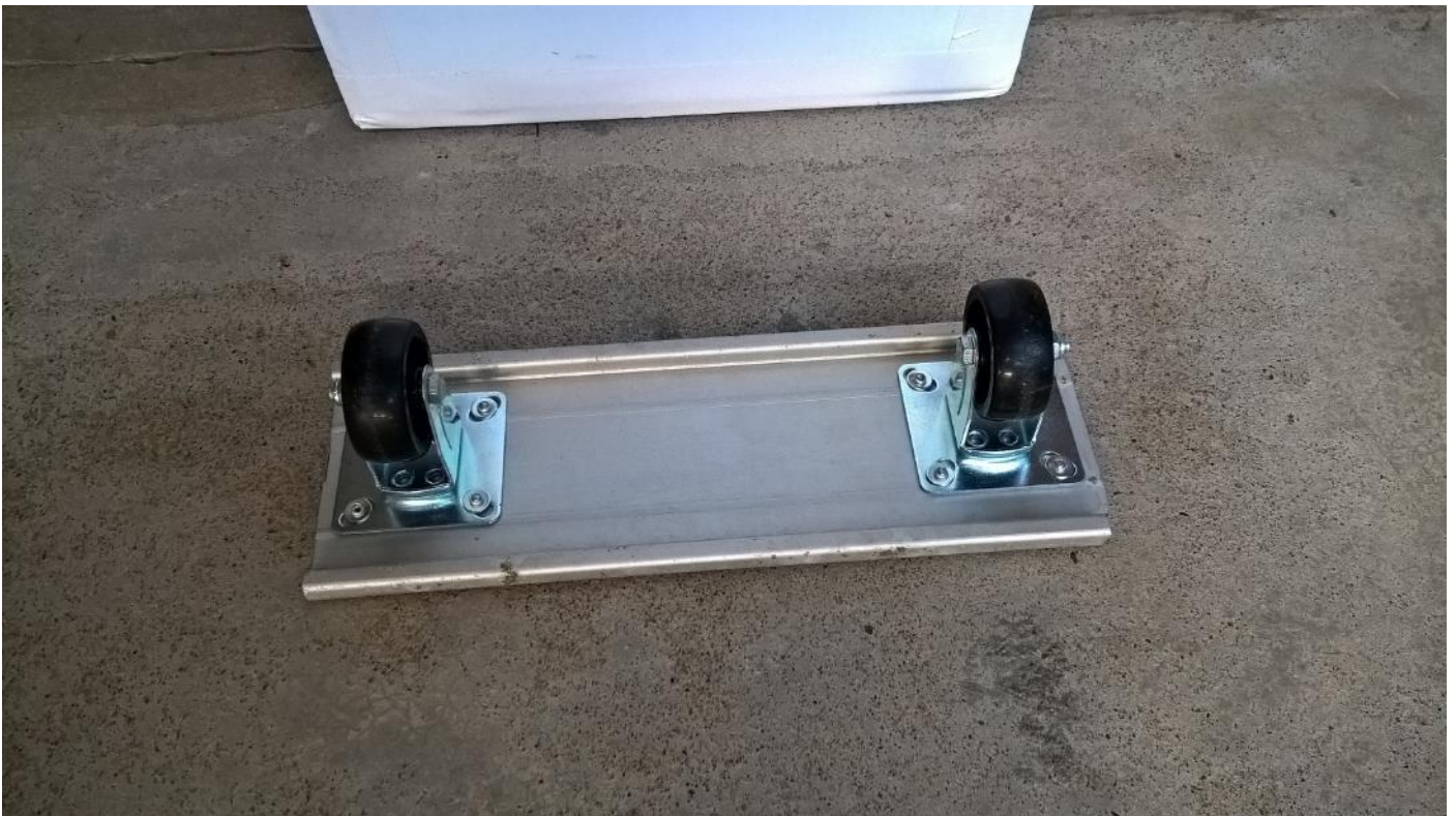
Figure 10: Trolley made from scrap aluminium channel and two wheels secured by rivets with washers.
