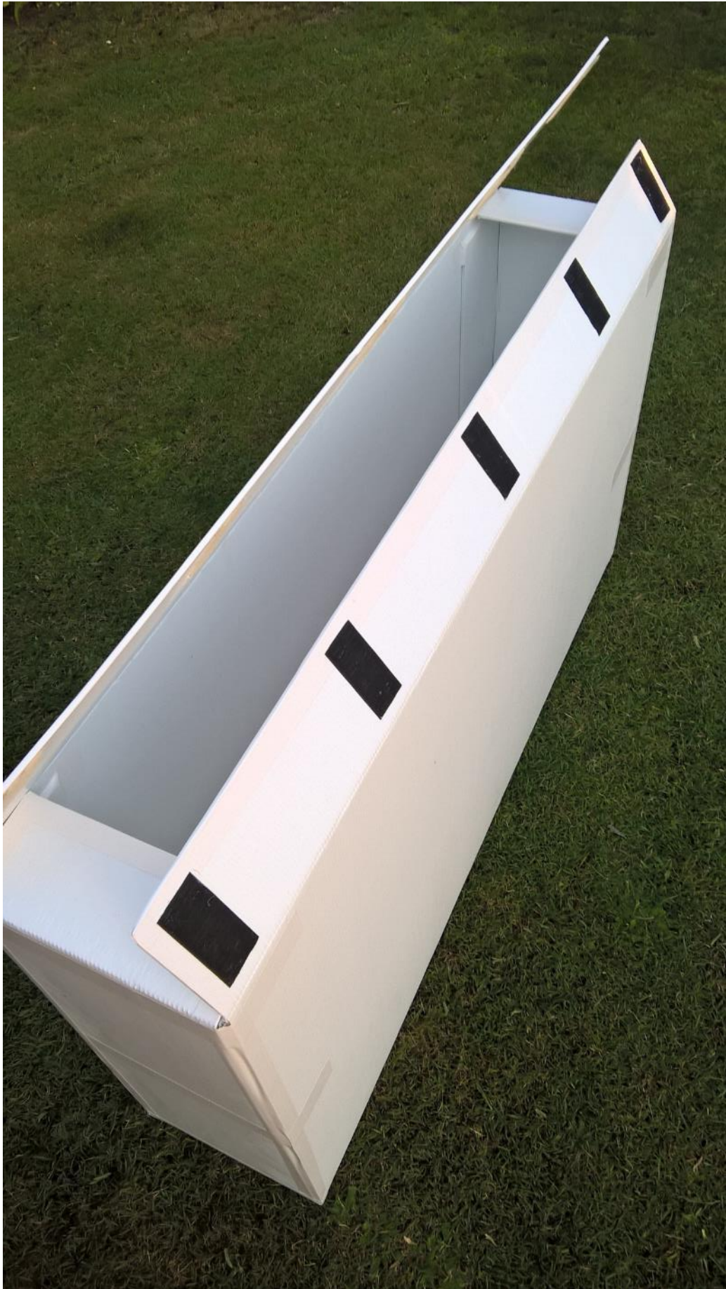
Figure 6: Finished box showing hook and loop fastener.
